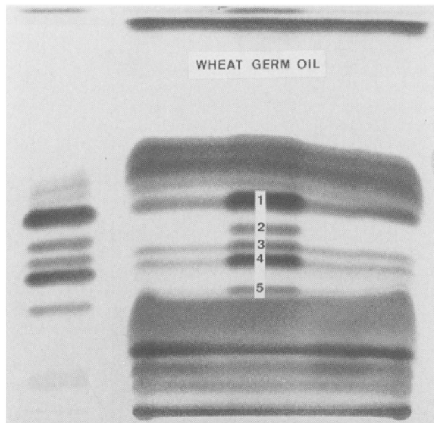
FIG. 1. Separation of individual tocopherols of 100 mg wheat germ oil on 0.25 mm TLC plate, silica gel 60 F 254, precoated, 20 x 20 cm. Solvent system— n -hexane/ethyl acetate 92.5:7.5 (v/v); 3 runs. Reference solution 0.1 ml on the left-hand edge and in the middle of the plate, containing 0.6% natural Mixed Tocopherols Concentrate + 0.04% synthetic \alpha -T 3 . Indicator: Emmerie-Engel reagent I, followed by respraying with Phosphormolybdic acid reagent II; heated 10 min 90 C. 1 = \alpha -T, 2 = \alpha -T 3 , 3 = \beta -T, 4 = \gamma -T, 5 = \delta -T. The oil does not contain \alpha -T 3 ; \gamma -T includes also \beta -T 3 . At the start: ASCP.
